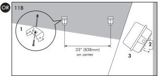
Insert hanging chain (not included) into "V" clip. Attach "V" clip to the base bracket.
