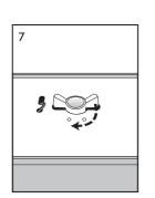
Rotate the locking pin 1/4 turn to secure lamp reflector.
